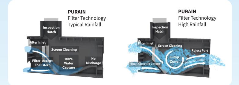
Using the unique jump filter design, **PURAIN** filters catch 100% of rainfall up to a certain flow rate. At higher flow rates, the filter is vigorously cleaned using what is called a hydraulic jump action. This leads to the highest overall water capture efficiency, regardless of geography. No other self-cleaning filter can make that claim.
